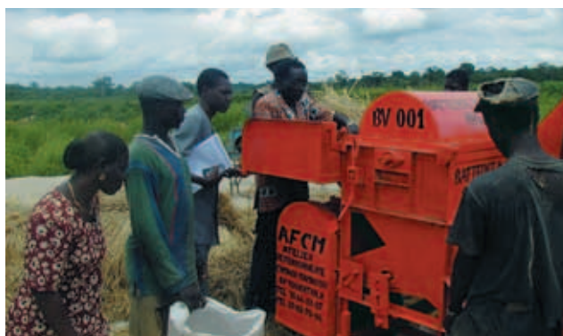
Proud owner of ANWAR BV 001, Lamine Coulibaly, operating the thresher–cleaner for farmers in the Lope perimeter
